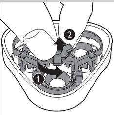
**3** Turn the wheel anticlockwise (1) and remove the retaining frame (2).
