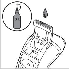
*Tip: Lubricate the trimmer teeth with a drop of sewing machine oil every six months.*
