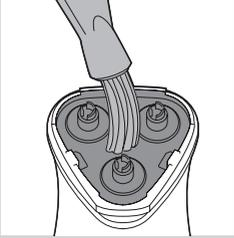
**4** Clean the inside of the shaving unit and the hair chamber with the cleaning brush.
