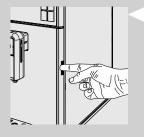
2 Press the button in the frame and open the service door.
