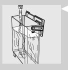
8 Empty the drip tray (internal) / (external). Press the "\sqrt{"} button.
