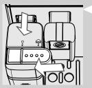
12 Insert the milk carafe dispenser back into position, scrolling it up to the "●" icon. Remove the milk carafe and empty it.
