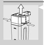
1 Press the release buttons to remove the top of the carafe.
