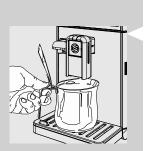
You need to perform a rinse cycle when using the machine for the first time. During this process, the coffee brewing cycle is activated and fresh water flows through the dispensing spout. This takes a few minutes.
