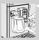
7 When the dispensing is complete, empty the container and place it back under the water dispensing spout.
