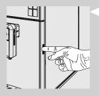
1 Press the button in the frame and open the service door.
