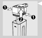
1 Press the release buttons to remove the top of the carafe.
