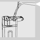
4 Remove the lid and fill the milk carafe up to the MAX level with fresh water.
