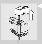
3 Lift the dispensing spout to remove it from the top of the carafe. The milk carafe dispenser is made up of five parts that must be disassembled. Each part is indicated by a capital letter (A, B, C, D, E) as shown in the figure below.
