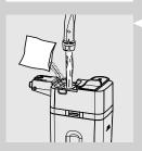
8 Pour one milk cleaner bag into the milk carafe. Fill the milk carafe with fresh drinking water up to the MAX level and then let the milk cleaner bag dissolve completely.
