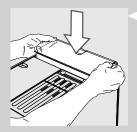
4 Insert the coffee bean hopper into its compartment as shown on the figure.
