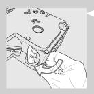
**13** When you reach the position shown in this figure, check that the two reference signs match and that the brew group is locked into position.
