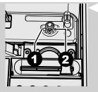
3 The reference marks in the coffee bean hopper compartment indicate the grind setting. There are 5 different grind settings to choose from position 1 for coarse grind - lighter taste to position 2 for fine grind bolder taste.
