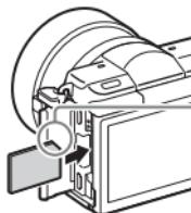
Ensure that the notched corner is faced correctly.
