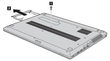
3 Remove the screw 3, then remove the optical drive bracket in the direction shown by arrow 4.
