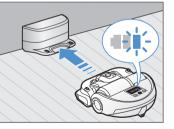
When the battery indicator blinks during cleaning, POWERbot will return to the charger to charge itself automatically.
