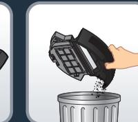
**EN** The robot must be emptied and cleaned after each use. Push the button on the backside of the robot and pull out the dust container. To empty it, flip off the cover.
