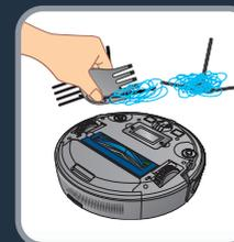
**EN** To clean the side brush, remove it and use a cleaning brush to clean the side brush and the entanglements in the slot of the side brush. Replace lateral brushes every 6 months.
