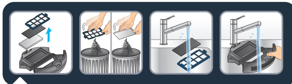
**EN** Clean the filter cover and the filter by tapping the back, holding it above a waste bin. Wash the foam filter, the filter cover and the dust catcher in clean water. Do not wet the fine dust filter (white filter). The filters must be cleaned at least once a week.
