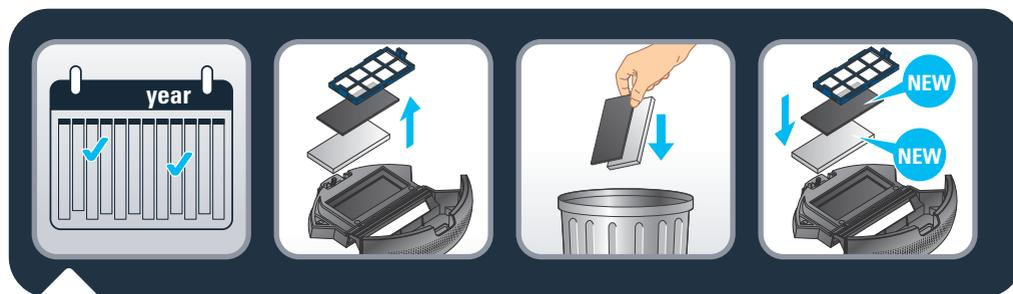
**EN** Every 6 months replace the fine dust and foam filter with new ones to maintain optimal performance.
