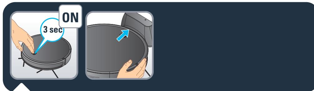
**EN** To charge the robot turn it on by pushing the on / off button for 3 seconds. Place the robot on the docking station: the charging plates on the robot must touch those on the docking station. Replace the robot on its charging base after use.
