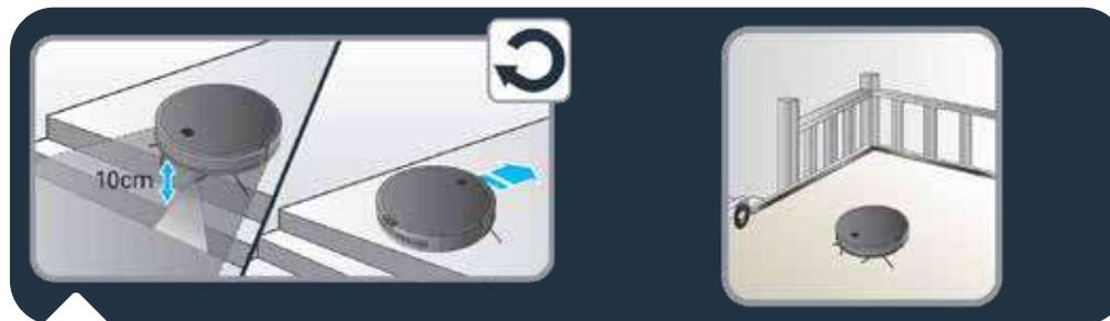
**EN** The robot has drop sensors to detect stairs and gaps. The robot will change direction when detecting them. In order to correctly detect the floor level difference, make sure there are no objects (bags, shoes...) on the floor next to gaps, stairs or on the stairs' steps. The step must be more than 10 cm away to be detected. If the area to be cleaned has stairs, a magnetic strip must be placed at the edge of a drop in order to prevent product damage and ensure safe operation.
