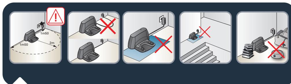
**EN** To place the docking station, make sure there is an empty area of 1.5m on each side and 2m in front of the docking station. Do not install the docking station near stairs. The cable must be tight. Always place the docking station on hard floor. Do not place the docking station on carpet.
