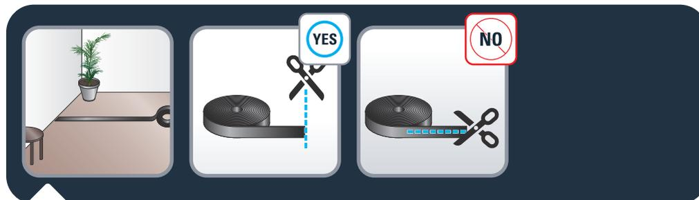
**EN** Should you like to restrict access of the robot to some areas, use the magnetic stripe. Put the magnetic stripe on the floor to mark a no-go zone for the robot. You can cut the magnetic stripe in pieces to adjust its length to your need. Please cut it only vertically and never along the stripe.
