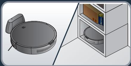
**EN** In order to extend the battery lifespan, always keep the robot charging on the docking station while not using it. If the robot is stored off/out of the docking station, make sure the robot is OFF and the battery is fully charged. Store the robot in a fresh and dry place. Please charge the robot every 3 months when you are not using it.
