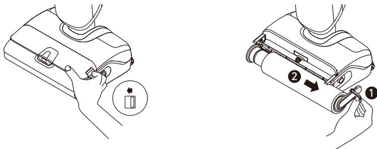
3. Clear any hair and debris caught on the roller brush with the provided cleaning brush. Rinse the roller brush and the cover with clean water and dry it completely.
