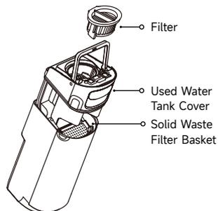
3. Pour out the used water, and clean the solid waste from the solid waste filter basket. Rinse with clean water. Use the provided cleaning brush to clean the inner walls of the tank.
