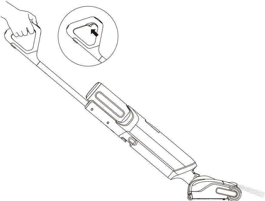
Note: Do not remove the brush cover while spraying hot water.
