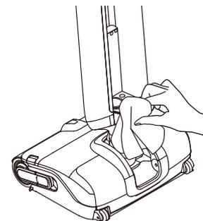
Note: Do not rinse the tube or the dirt sensor.
