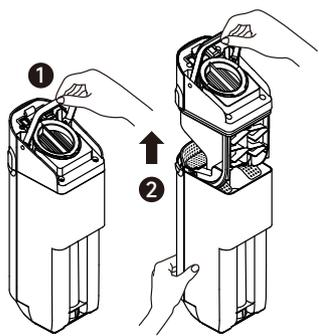
3. Pour out the used water, and clean the solid waste from the solid waste filter basket.
