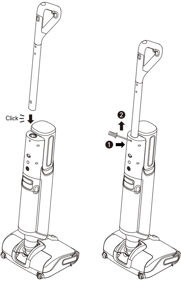
Note: To disassemble, extend a hard object into the hole of the appliance as indicated to press in the contacts and pull the handle upwards at the same time.
