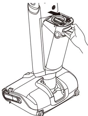
2. Pull up the used water tank cover handle, lift off the cover. Remove the filter.
