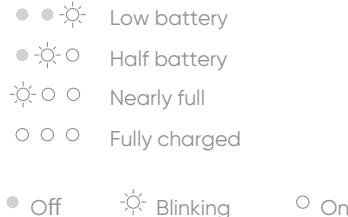
Note: Once the vacuum is fully charged, the indicator will turn off after 5 minutes, and the vacuum will enter the energy-saving mode.
