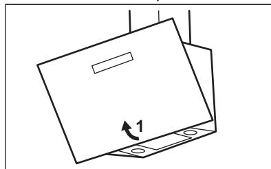
2. Press the handle of the mounting clip on the filter panel underneath the hood.
