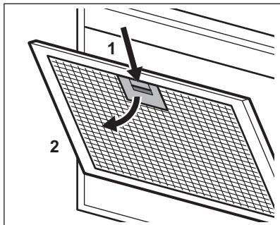
3. Slightly tilt the front of the filter downwards, then pull.
