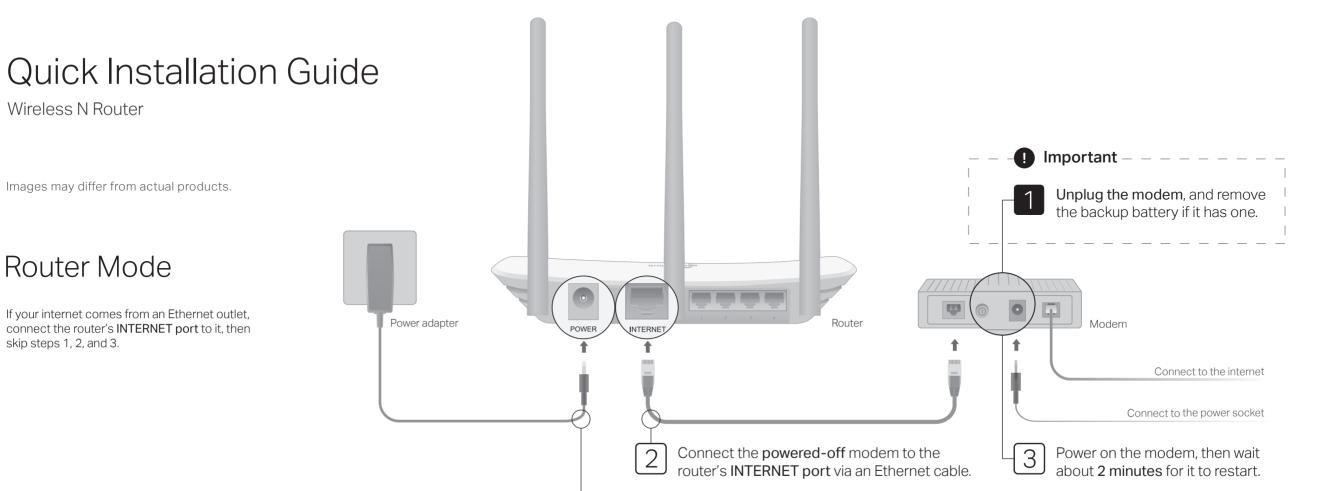
Connect the power adapter to the router.
