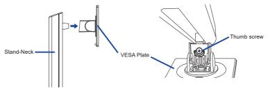
② Install the Stand-Base to the Stand-Neck and then tighten the 'thumb screw' to secure them.
