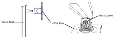
② Install the Stand-Base to the Stand-Neck and then tighten the 'thumb screw' with the provided screwdriver to secure them.
