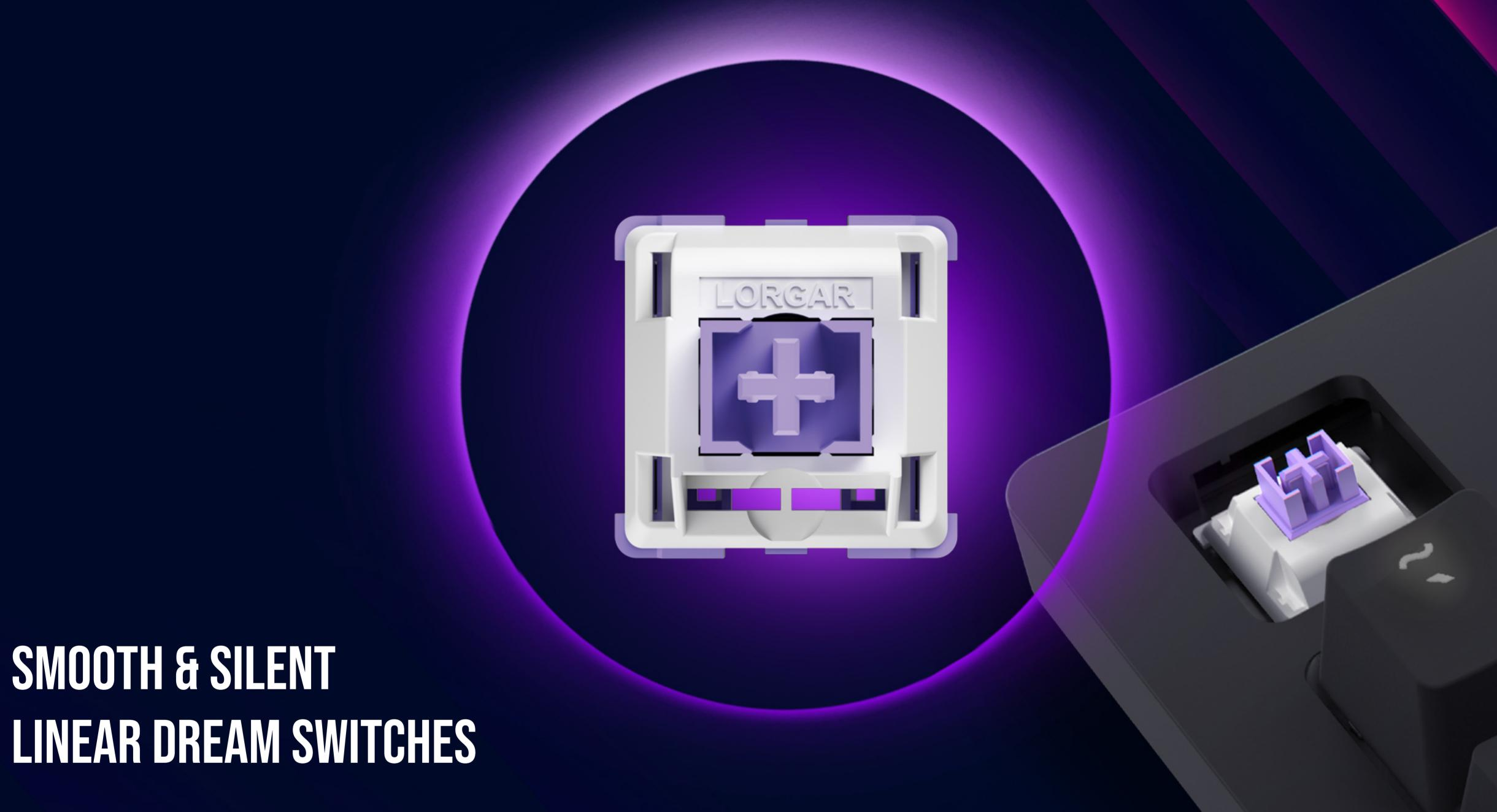
These Dream Switches can withstand 50 million cycles, making them highly dependable. With the balanced actuation force of 40 grams, no accidental input is expected, and the actuation point of 2mm within 4mm of travel distance gives you a reaction advantage in-game.
