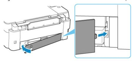
**9.** Insert the coin screw into the screw hole and turn it clockwise to secure.
