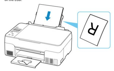
7. Slide right paper guide to align with both sides of paper stack.
