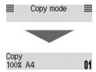
When the **COPY** button, **SCAN** button, or **Setup** button is pressed, the display switches to copy mode, scan mode, or setup menu screen.
