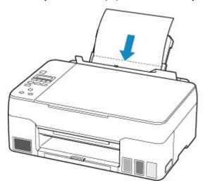
After loading paper on the rear tray, the paper information registration screen for the rear tray appears on the LCD. Select **A4** or **Letter** for **Size**:
