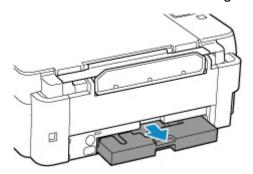
6. Lift the maintenance cartridge a little and pull it out.
