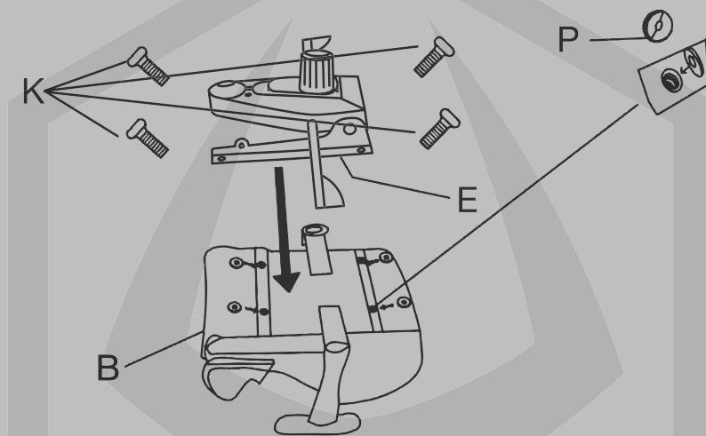
5. Place the seat assembly onto the multi-functional seat control base by inserting the gas lift cylinder into the center hole in the seat control base. Make sure the seat assembly is firmly pressed down into place before using the chair.
