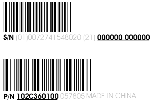
Figure 1–1 Typical Serial Number and 102 Part Number Arrangement
