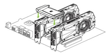
2-way SLI configuration: Install your second GeForce GTX 1080 graphics card into the outer PCI Express x16 slot (the outer slot is the one farthest away from the CPU).
