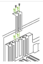
Remove two adjacent slot covers that corresponds to the PCI-Express slot you are installing the GeForce GTX graphics card in.
