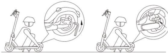
If you feel the brakes are too tight, use the hex wrench counter-clockwise to loosen the screws on the pressure plate on the disc brake seat. Release the brake line to shorten slightly the exposed length and tighten the screws of the pressure plate. If you feel that the brake is too loose, release the screws on the pressure plate, drag the brake cable to slightly lengthen the length and then lock the screws on the pressure plate.
