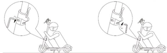
If you feel that the front bar is not tight enough, use the hex wrench to tighten the two screws in the folding mechanism.
