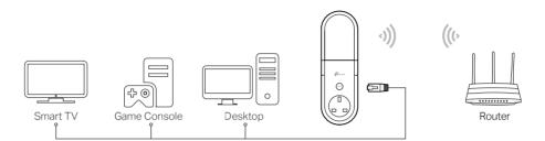
By default, the Ethernet port of the extender is connected to the 5GHz wireless netwok.
