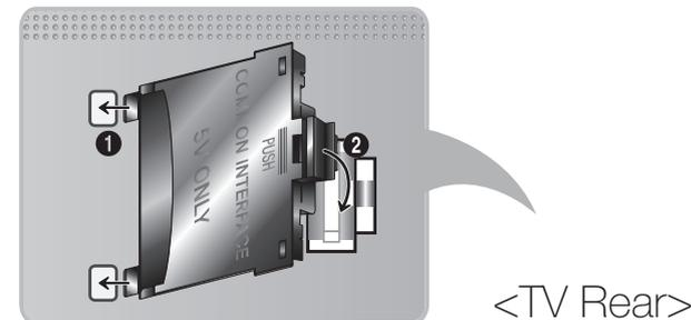
**1.** Insert the CI CARD Adapter into the two holes on the product **1**.
